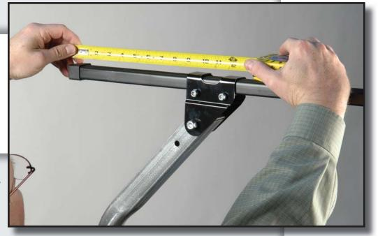
15. Center the loadbars by measuring that the same length of bar extends past the bracket on each side.
