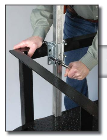
9. Assemble the bottom plates as shown using the square U-bolts and nuts, no washers here.
