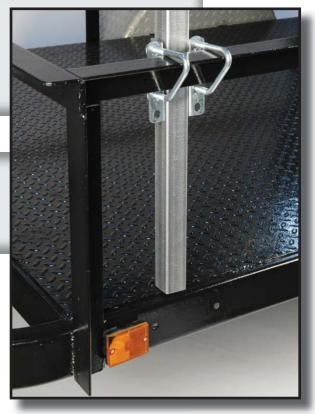
8. Measure that the uprights are in the same place on both sides of the trailer, then fully tighten all the U-bolts.
