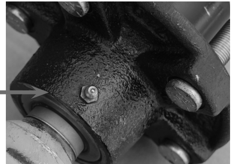
Integrated zerk fitting on the backside of the hub
