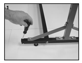
. Remove and discard the two plastic end caps from the rear side of the Frame Legs (A) . See image 1.
